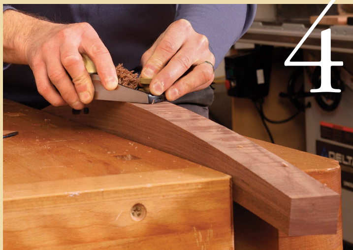
Block plane fairs a curve. To smooth a convex curve, continuously adjust the angle of the sole so the area just ahead of the blade rides the workpiece during the whole cut. Some very shallow concave curves can also be smoothed with the block plane, provided it is held askew.
