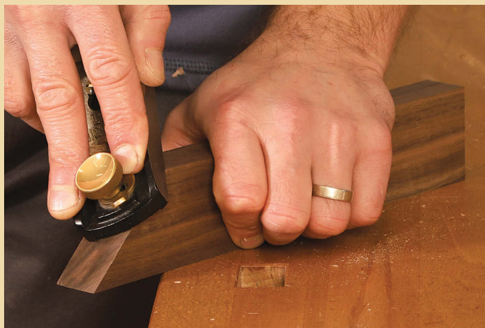
Fairing a miter. Rather than using a clamp to hold a mitered workpiece, Korsak holds it on edge with one hand and planes with the other. He does the same to plane end grain on most square-cut boards, steadying them on one edge with one hand while planing in a downstroke with the other.
