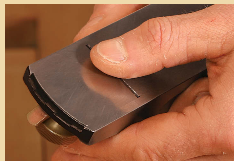
Final flushing. Using a second block plane, Korsak sets the cambered blade to take a very light cut (above) and finishes flushing the edging with several passes (left). The cambered blade lets him precisely focus the cut and avoid planing the adjacent veneer.
