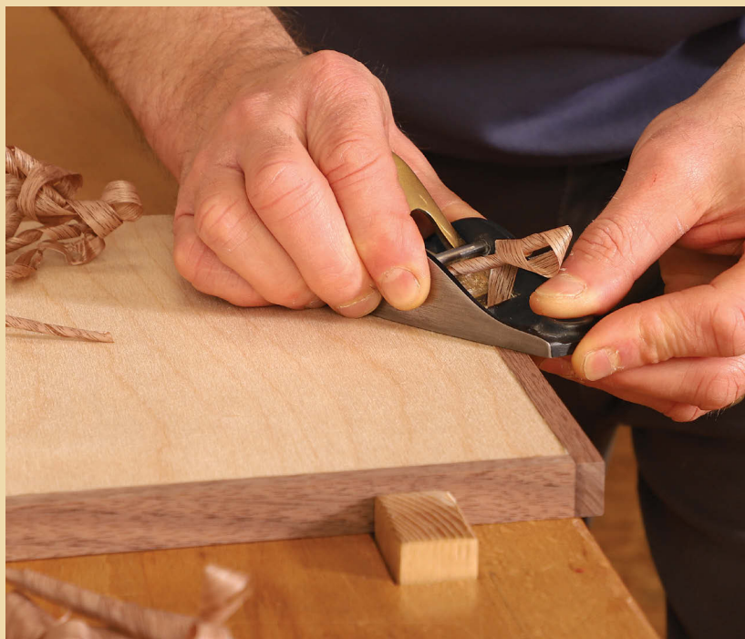
Flushing in two steps. Korsak uses two block planes to flush solid edging to a veneered panel. Here he takes a series of coarse shavings with the first block plane, stopping when the edging is about \frac{1}{64} in. proud of the panel.
