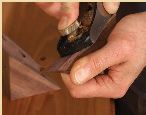
Fine tool for odd jobs. With its small size making one-handed operation easy, the block plane is handy for smoothing parts that are hard to clamp (left) and areas that are delicate or hard to reach (above).
