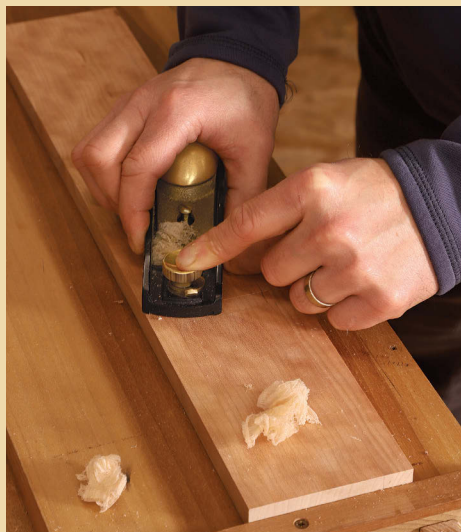
A little smoother. With a razor-sharp cambered blade set for a fine cut, a block plane can prepare a surface for finishing every bit as well as a smoothing plane. Korsak uses a block plane for smaller surfaces and a smoothing plane for larger ones.
