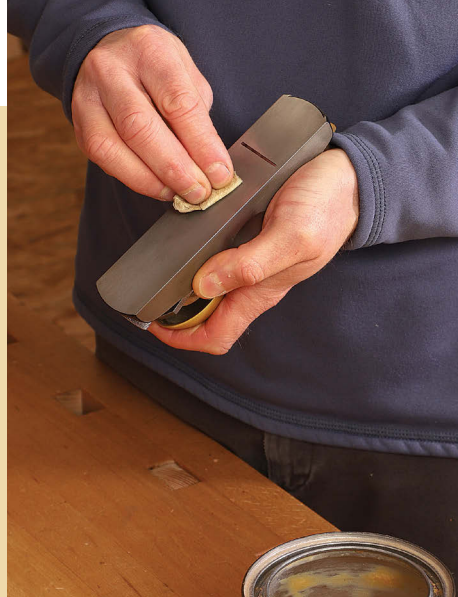
Wax up. Unless the surface he's smoothing will be glued (like some miters), Korsak waxes the sole of his block plane before planing end grain to minimize friction.
