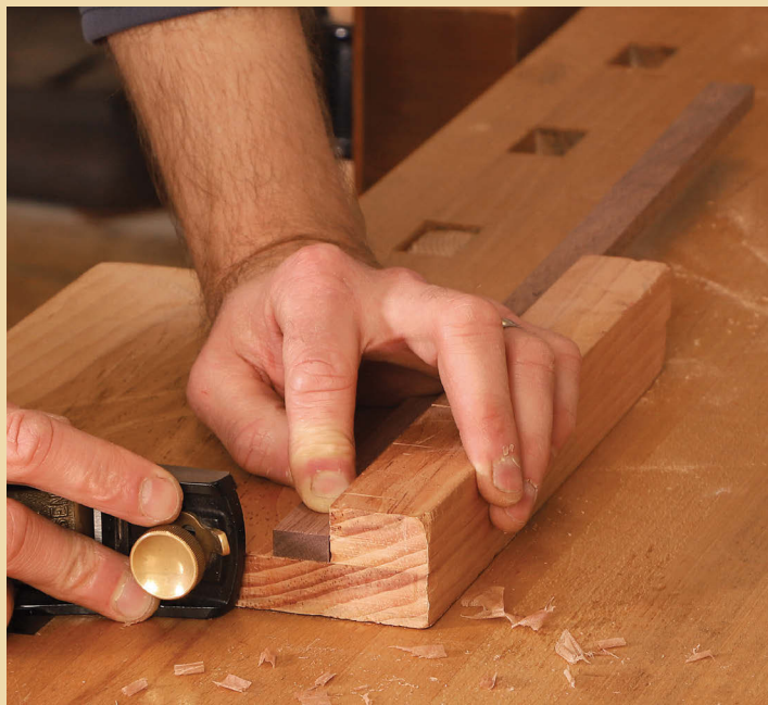
A hook helps with tiny parts. To smooth the end grain of very small workpieces, Korsak cradles the part in a bench hook and uses his block plane on its side.
