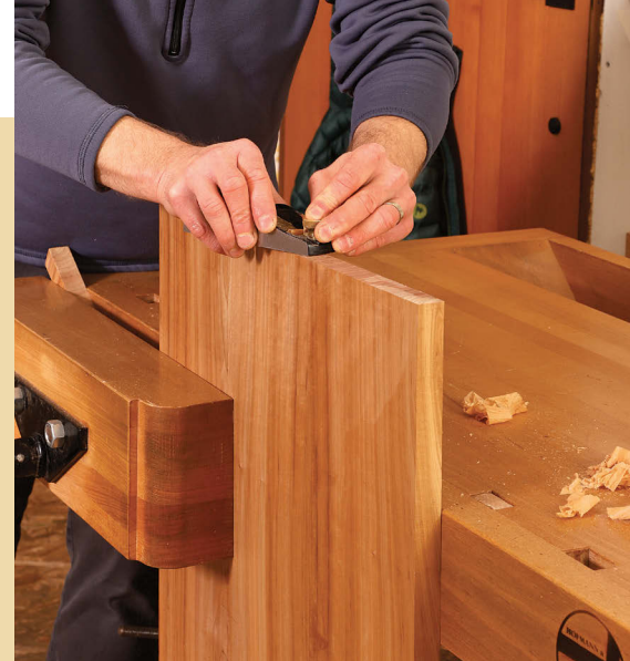
Use a vise for a wide board. When planing the end grain of wide boards like this one, Korsak fixes them in a vise.
