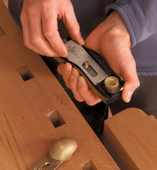
Swap out the iron. Korsak likes a freshly sharpened high-angle iron for end grain.
