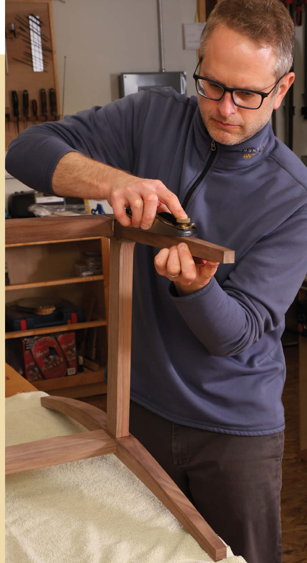
Fine tool for odd jobs. With its small size making one-handed operation easy, the block plane is handy for smoothing parts that are hard to clamp (left) and areas that are delicate or hard to reach (above).
