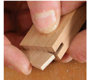
Runners get an open mortise for a slip tenon. Cut these slots using the same blade you used to groove the aprons. Position the slots so the tops of the drawer runners are flush with the bottom of the drawer openings.
