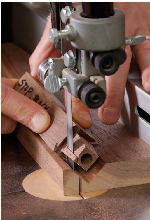
Slicing on the bias. With a stop block screwed in place behind the blank, Korsak makes tapered stopped cuts with each of the blank's four corners in turn cradled in the V-groove.
