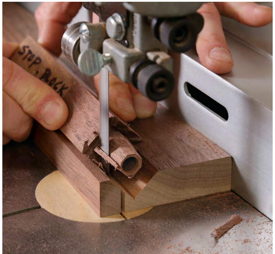
Slicing on the bias. With a stop block screwed in place behind the blank, Korsak makes tapered stopped cuts with each of the blank's four corners in turn cradled in the V-groove.
