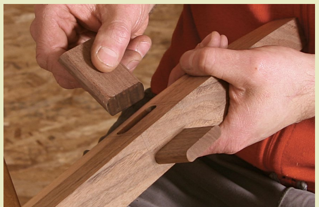
To maximize the length and strength of the slip tenons, Korsak glues them into intersecting mortises, being sure the miters meet. Once the glue cures, he proceeds with the full assembly.
